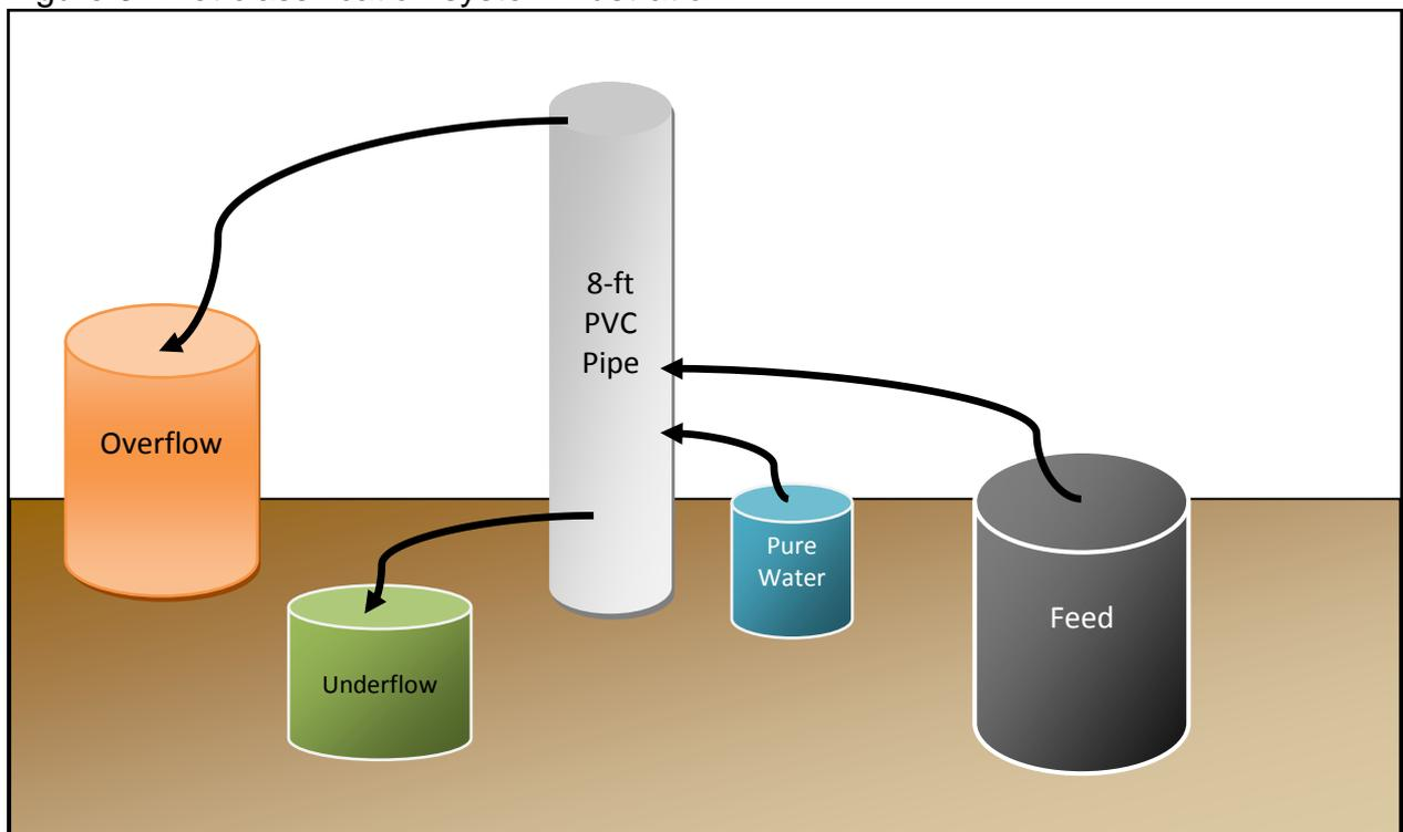
The hydraulic classification was used due to its potential to reduce the naturally high free lime content of GFA while simultaneously obtaining a large sample of finer particle size.
