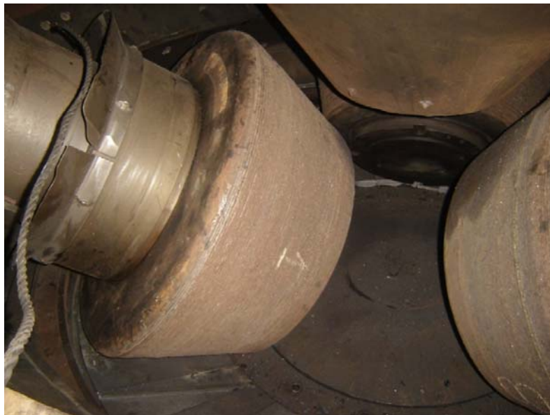
Picture 3: A Grinding Roll View Inside the Mill
