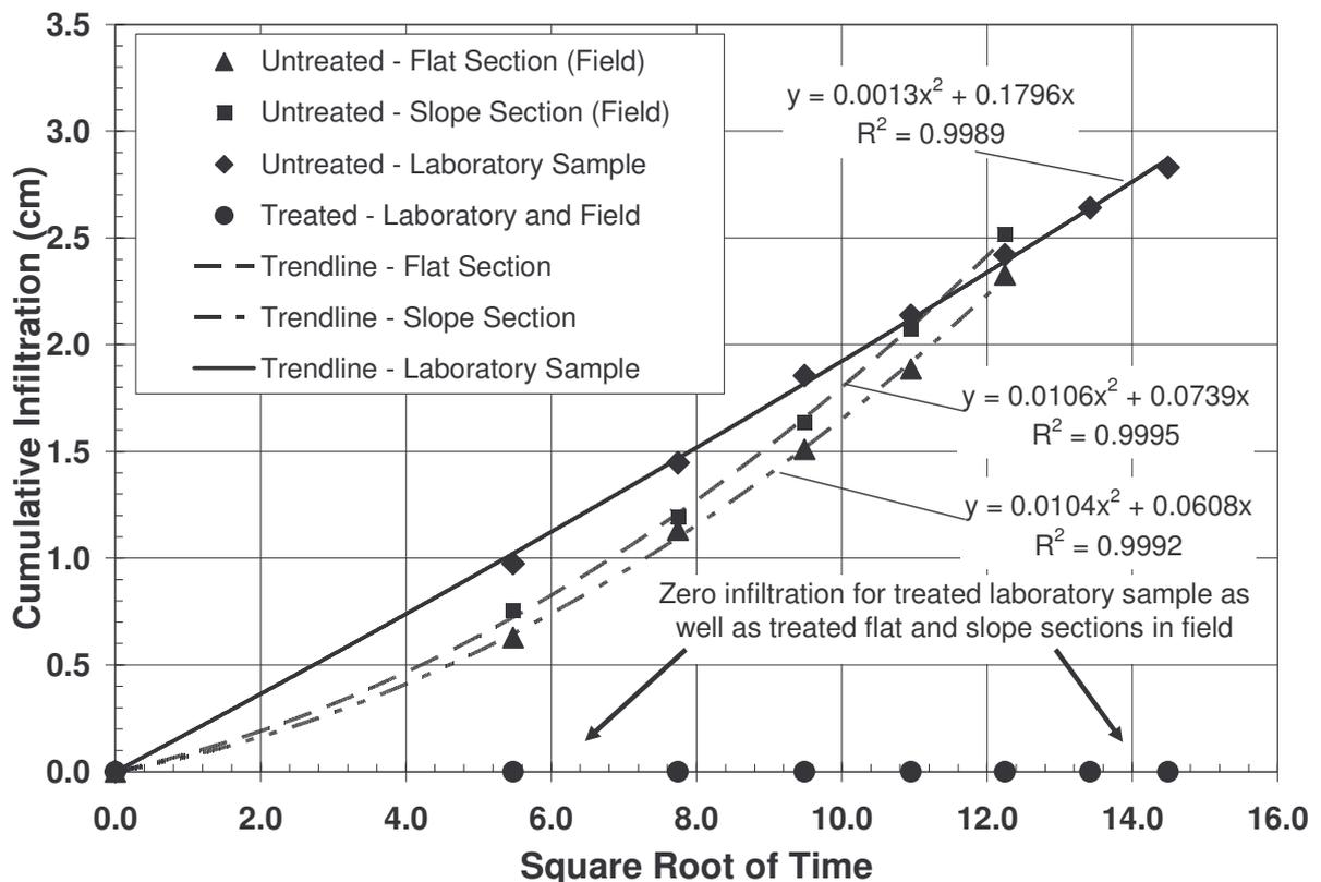
Figure 2. Infiltrometer results for laboratory and field samples
