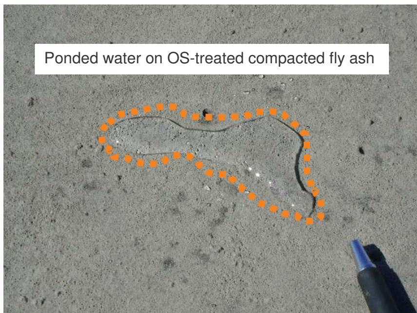
Figure 3. Development of hydrophobicity on OS-treated flat section of field site (typical)
