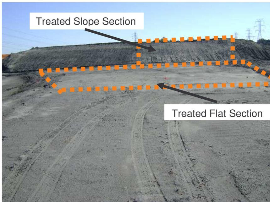
Figure 1. Treated and untreated sections of field test site (ash monofill).
