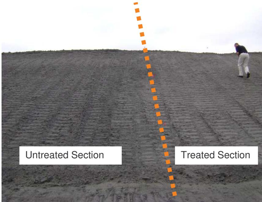
Figure 4. Example of slope after precipitation event – right side remained dry, as evidenced in part by a lighter color (from top to bottom) and verified on-site.
