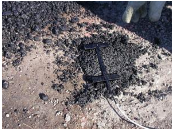
Figure 4: Placement of the strain gauge at the top of the FDR layer in Delaware County.
