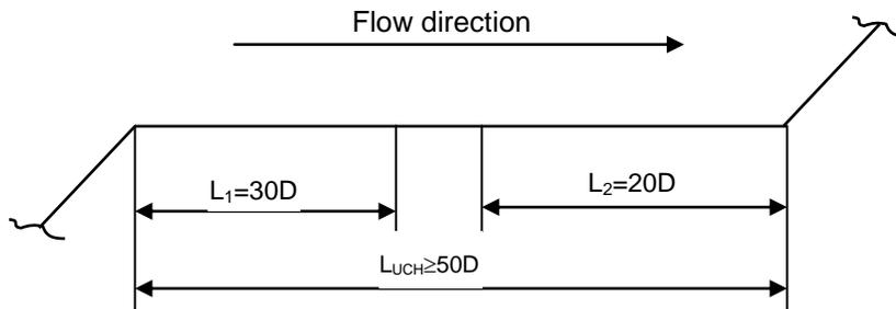
Fig.2. Configuration of the pneumatic ash pipeline section:  $L_{uch}$  — length of the rectilinear horizontal (vertical) section at the complex pneumatic ash pipeline route;  $L_1$  — length of the aerodynamic stabilization section of the ash-air flow after the local resistance;  $L_2$  — the same, but before the local resistance.
