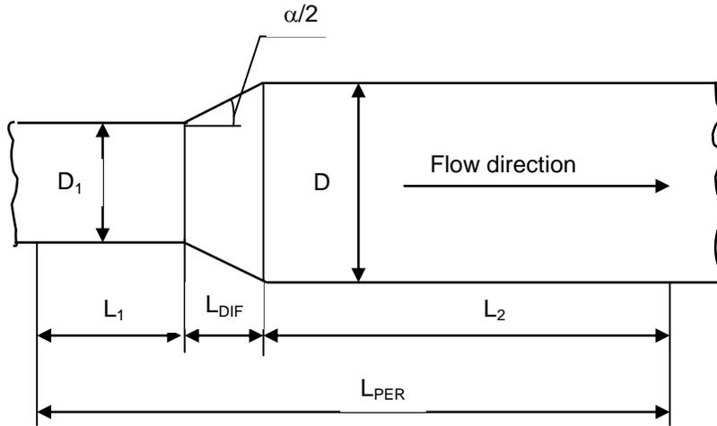
Fig.1. A form of the diffuser transiting from the smaller diameter of the stepped pipeline to the greater one:  $L_{PER}$  — total transition length with sections of aerodynamic stabilization of the dust-air flow;  $L_{DIF}$  — diffuser transition length;  $D_1$  and  $D_2$  — inner pipeline diameters before and after diffuser transition;  $L_1$  and  $L_2$  — aerodynamic stabilization sections of the dust-air flow before and after diffuser transition;  $\alpha$  — diffuser transition angle.
