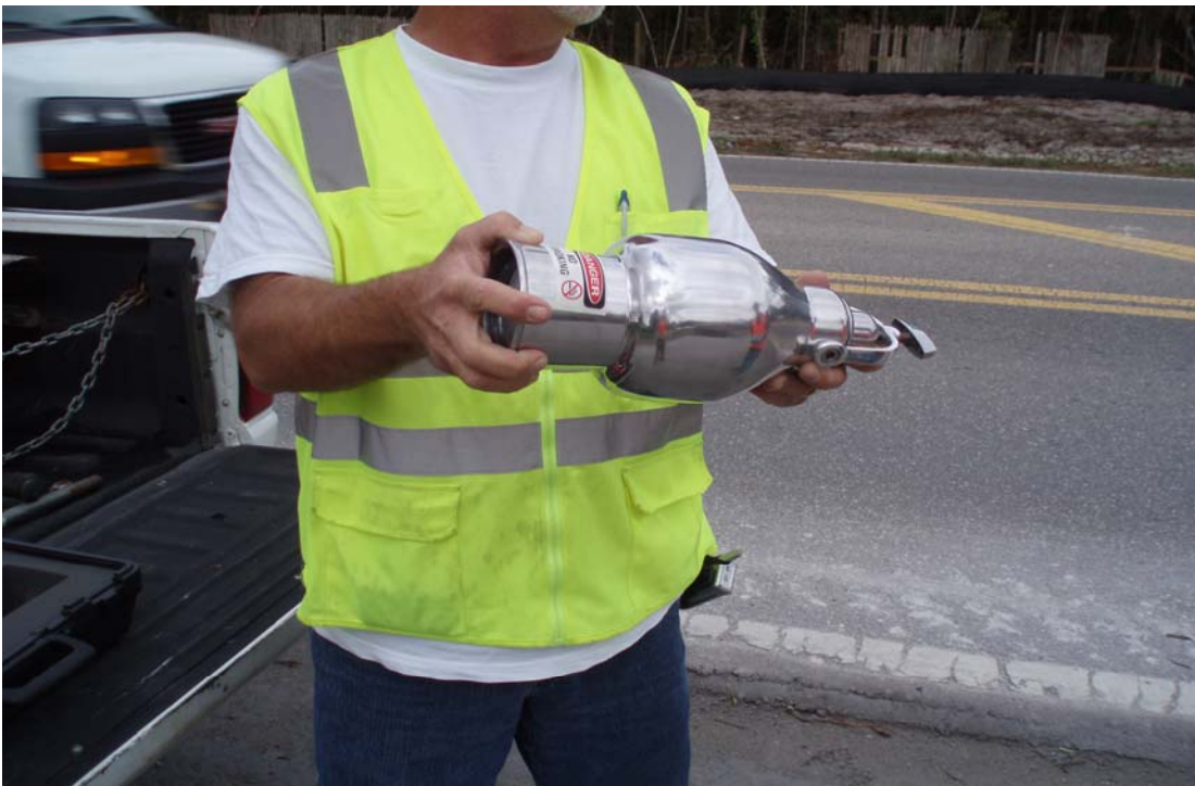
Figure 11. Moisture Content Testing with the Speedy Moisture Content Gage.
