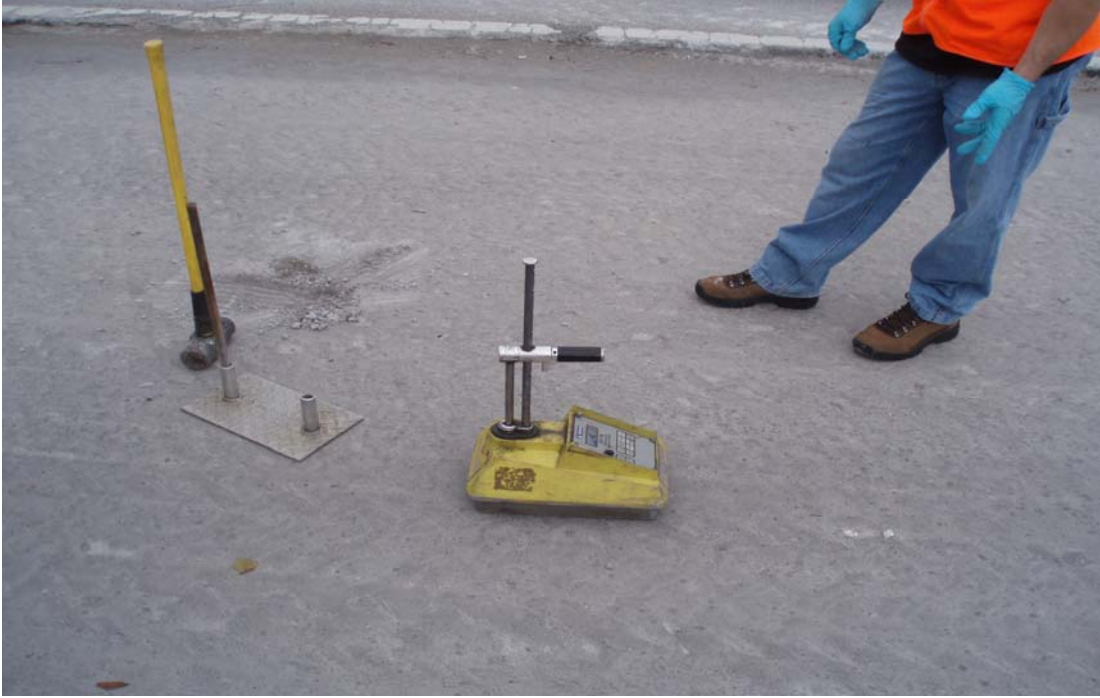
Figure 10. In-Situ Density Testing with the Nuclear Density Device.
