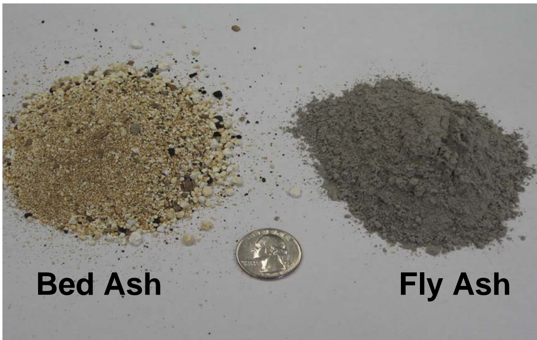
Figure 2. JEA's CFB By-Product Dry Bed Ash (left) and Dry Fly Ash (right)
