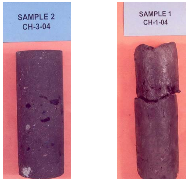
Figure 5 Condition of Grout within the Frazee Mine The Winding Ridge Project Friendsville, Maryland
