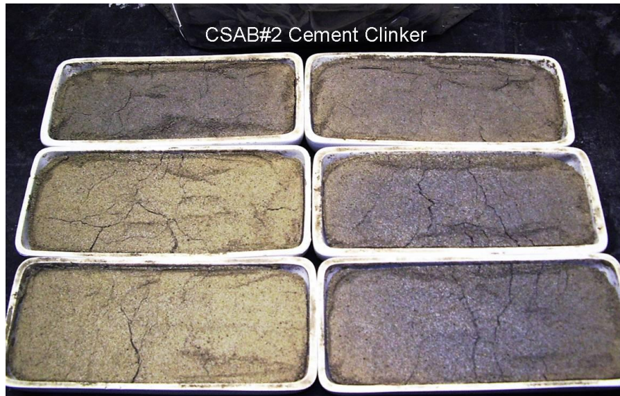
Figure 2. Synthesized CSAB#2 cement clinker produced with Gilbert CFBC spent bed materials. The clinker was fired at 1250°C in zirconia combustion for one hour.
