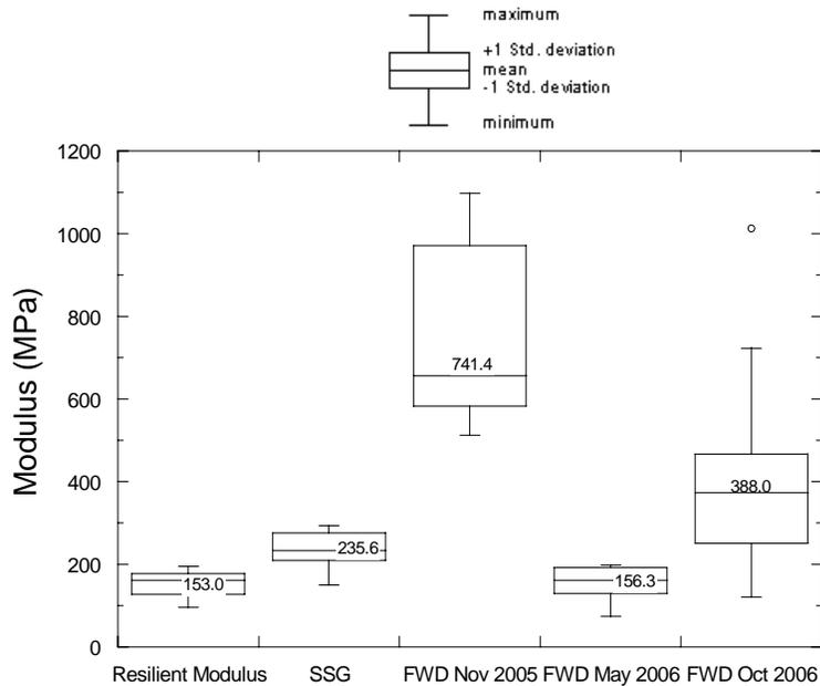
Fig. 4. Moduli obtained from different procedures and at different times
