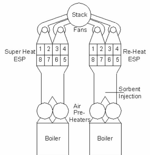
The sorbents were simply injected into the plant flue gas from lances ahead of the existing particulate collector. There, in the second of two that they have before being captured by the ESP, they adsorb and sequester the gas-phase elemental and oxidized mercury from the flue gas. To insure good duct coverage and mixing with the flue gas, an iterative design process for optimal lance placement was used at Crawford utilizing computational fluid dynamic modeling.
