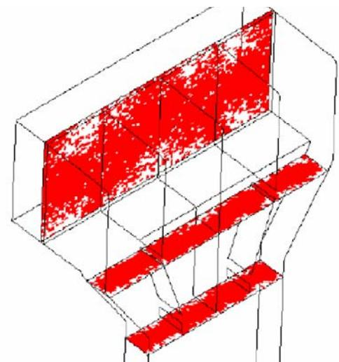
Right: The sorbent particle distribution at the ESP entrance plenum from the CFD model with an optimized injection design of 10 lances.
