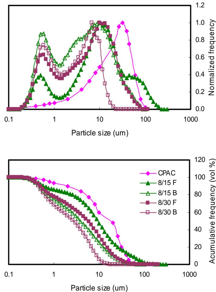
Figure 4. Particle size distributions of C-PAC<sup>™</sup> and fly ash measurements by Headwaters.
