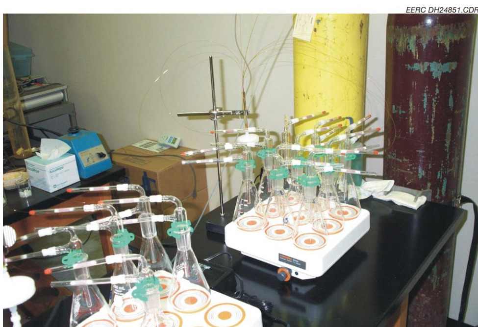
Figure 1. Microbiologically mediated mercury vapor-phase collection apparatus utilizing a stir plate to facilitate mixing.
