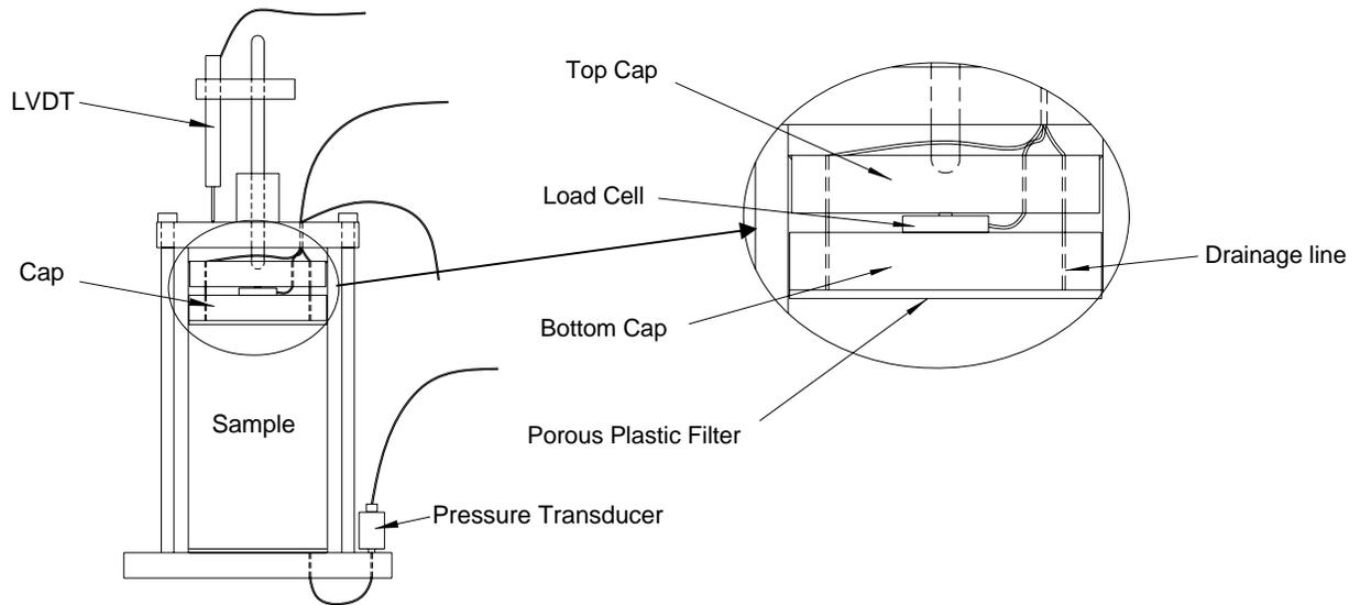
Figure 3 Schematic Cross Section of Instrumented Consolidation Chamber
