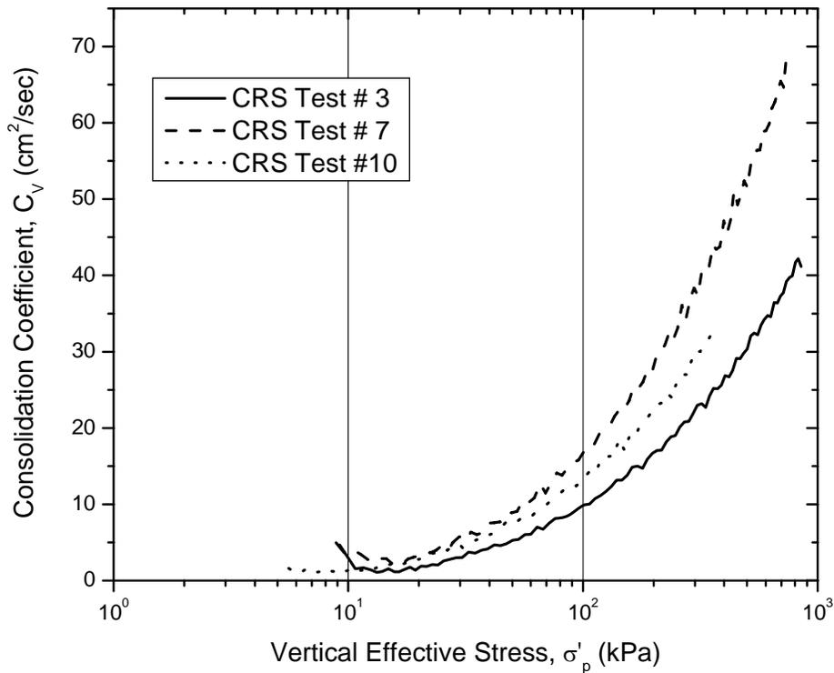
Figure 7 Coefficient of Consolidation  $C_v$  vs. Stress Level
