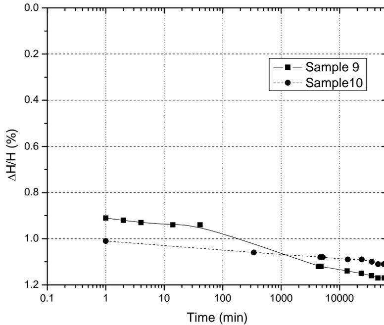
Figure 9 Secondary Compression Curves from Oedometer Tests
