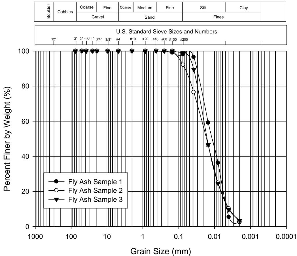
Figure 1 Grain Size Distribution of Fly Ash
