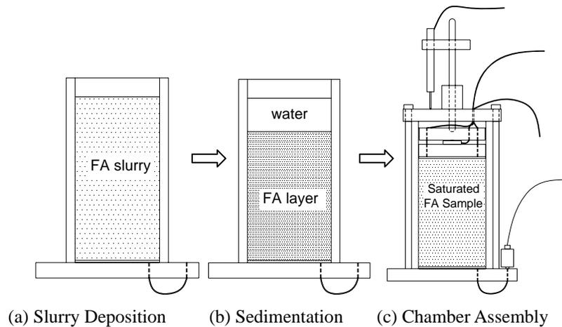
Figure 2 Schematic of Sample Preparation Methodology
