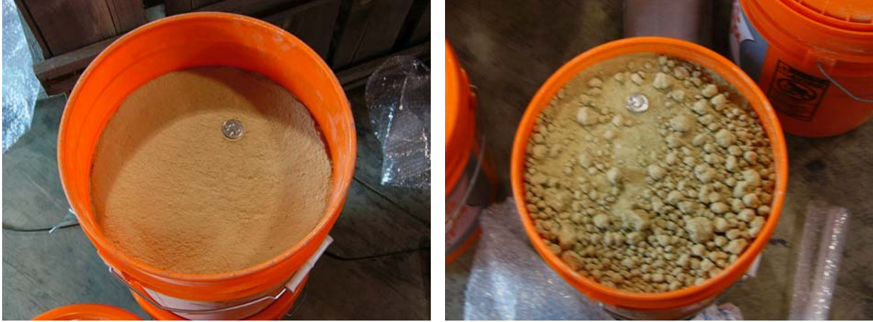
Figure 1. Photos Showing Fresh (left) and Moisture Conditioned (right) Spray-Dryer Ash
