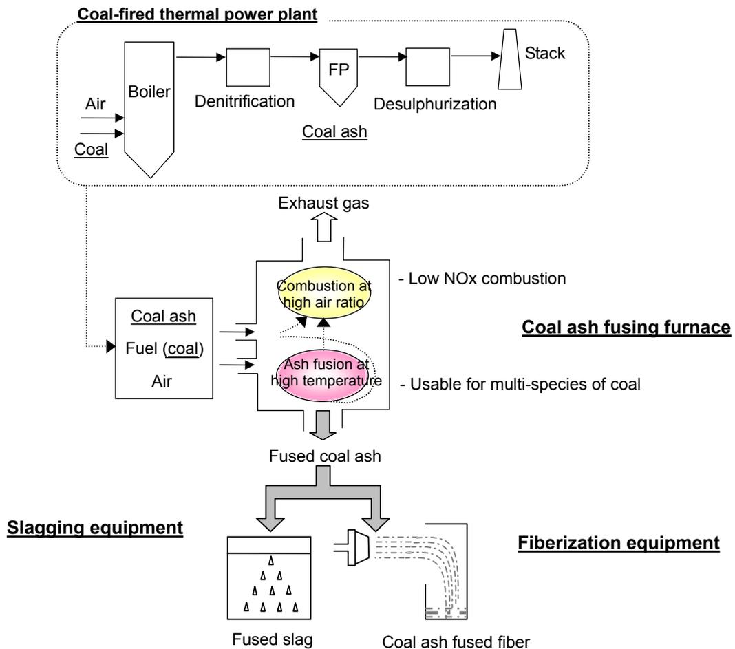
Fig. 2 Concept of the coal ash fusing and fiberization system
