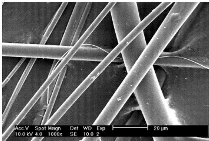
**Photo 1 Coal ash fused fibers produced as a test product**
