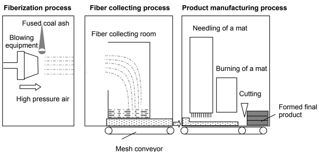
**Fig. 4 Structure of the fiberization system**
