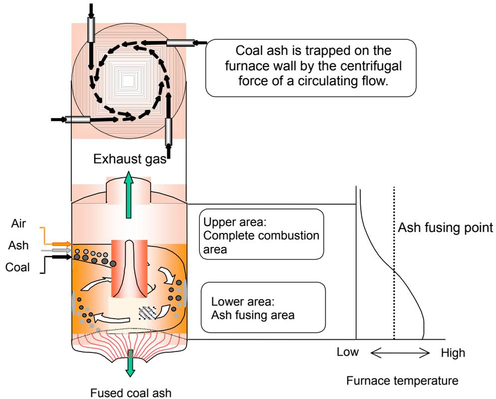
**Fig. 3 Description of the circular combustion type fusing furnace**
