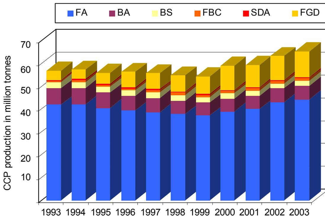
FGD = flue gas desulphurization gypsum; SDA = spray dry absorption product; Other = fly ash and slag from coal gasification, sulfur, sulfuric acid; FBC = fluidized bed combustion residues; BS = boiler slag; BA = bottom ash; FA = fly ash
