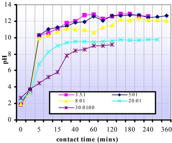
**Figure 2: Variation of pH with contact time (mins) for various AMD:FA ratios for Brugspruit (2) AMD and Matla fly ash react**
