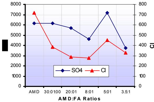
Figure 11: Concentration of SO4, Cl (mg/l) in final process waters with AMD:FA ratio for Brugspruit (2) and Matla fly ash
