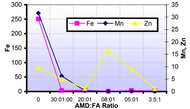
Figure 7: Concentration of Fe, Mn, Zn (mg/l) in final process waters with AMD:FA ratio for Brugspruit (2) and Matla fly ash
