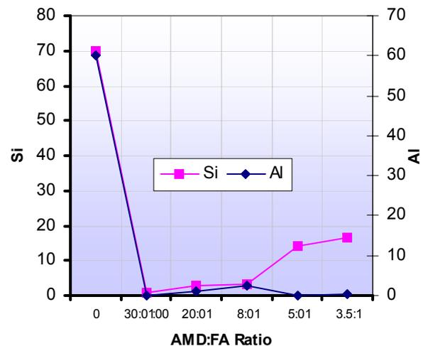
Figure 8: Concentration of Si, Al (mg/l) in final process waters with AMD:FA ratio for Brugspruit (2) and Matla Fly ash.
