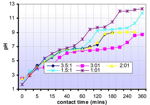
**Figure 4: Variation of pH with contact time (mins) for various AMD:FA ratios for Bank AMD and Matla fly ash.**
