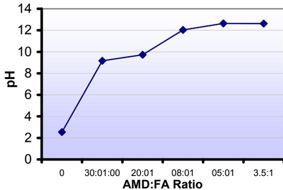
Figure 5: Change in pH of final process water with AMD: FA ratio for Brugspruit (2) and Matla fly ash
