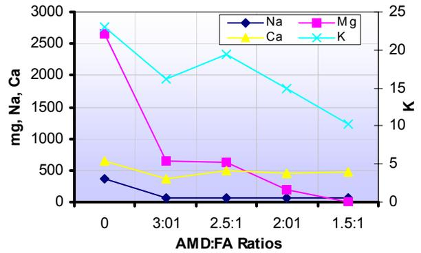
Figure 13: Concentration of Na, K, Mg, Ca (mg/l) in final process waters with AMD:FA ratio for Navigation and Matla fly ash
