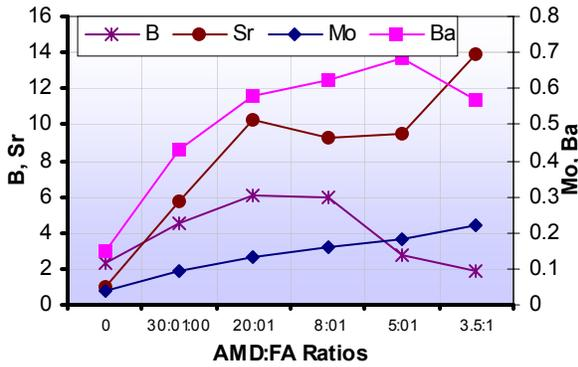
Figure 10: Concentration of B, Sr, Mo, Ba (mg/l) in final process waters with AMD:FA ratio for Brugspruit (2) and Matla fly ash
