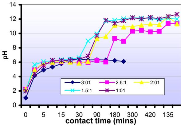
**Figure 1: Variation of pH with contact time (mins) for various AMD: FA ratios for Brugspruit (1) AMD and Matla fly ash reactions**
