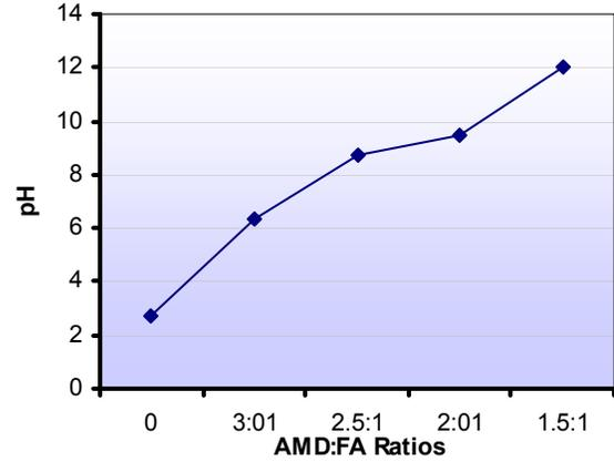
Figure 12: Change in pH of final process water with AMD:FA ratio for Navigation and Matla fly ash
