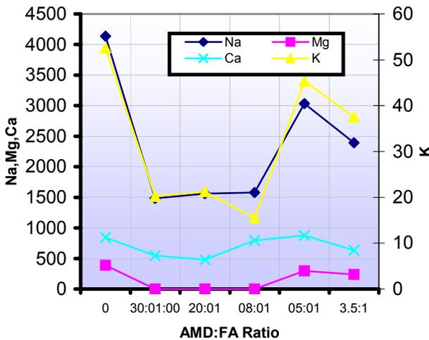
Figure 6: Concentration of Ca, Na, Mg, K (mg/l) in final process waters with AMD:FA ratio for Brugspruit (2) and Matla fly ash
