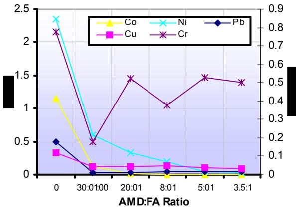
Figure 9: Concentration of Co, Ni, Pb, Cu, Cr (mg/l) in final process waters with AMD:FA ratio for Brugspruit (2) and Matla fly ash
