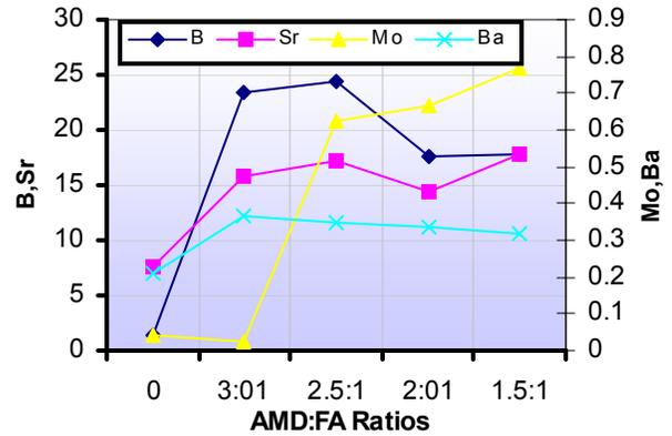
Figure 17: Concentration of B, Sr, Mo, Ba (mg/l) in final process waters with AMD:FA ratio for Navigation and Matla fly ash
