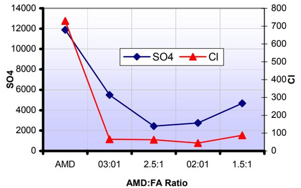
Figure 18: Concentration of  $SO_4^{2-}$ ,  $Cl^-$  (mg/l) in final process waters with AMD: FA ratio for Navigation and Matla fly ash
