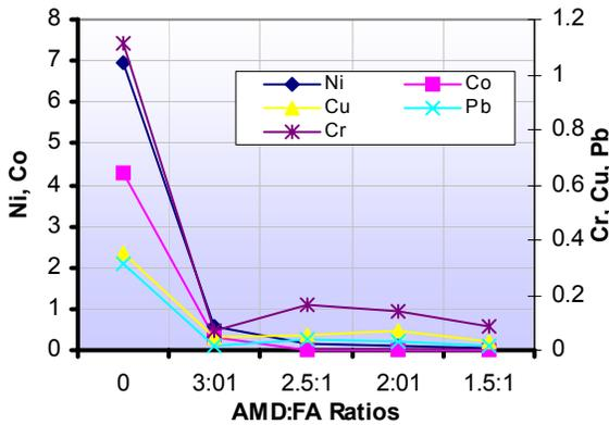
Figure 16: Concentration of Ni, Co, Cu, Pb, Cr (mg/l) in final process waters with AMD: FA ratio for Navigation and Matla fly ash
