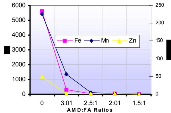
Figure 14: Concentration of Fe, Mn, Zn (mg/l) in final process waters with AMD:FA ratio for Navigation and Matla fly ash
