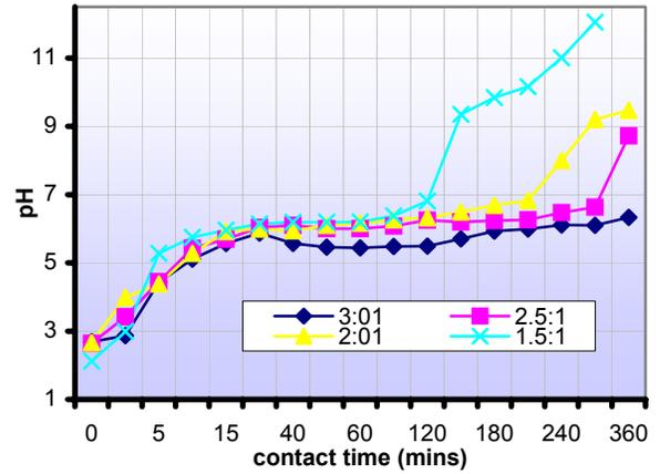
**Figure 3: Variation of pH with contact time (mins) for various AMD: FA ratios for Navigation AMD and Matla fly ash reactions**
