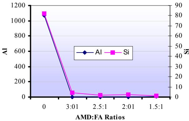
Figure 15: Concentration of Al, Si (mg/l) in final process waters with AMD: FA ratio for Navigation and Matla fly ash
