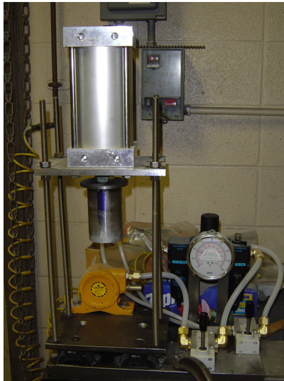
Figure 1. Laboratory-scale pneumatic piston with vibrator.
