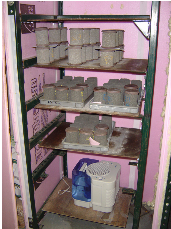
Figure 4. Capped cylinders in curing cabinet.
