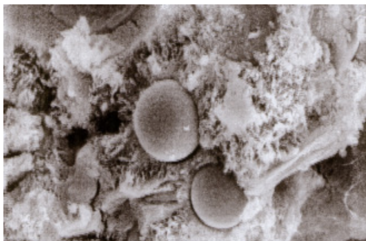
Figure 8 Dense C-S-H Gel Around a Fly Ash Sphere After 6 Months
