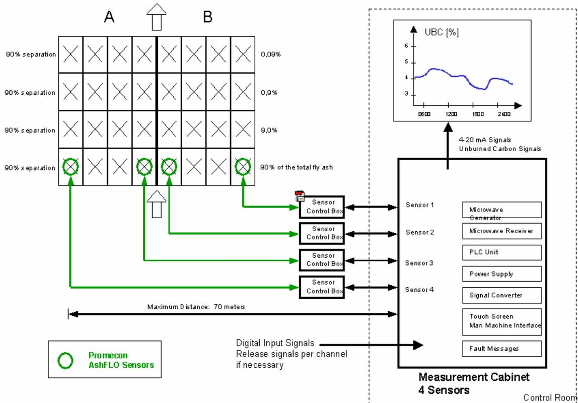
Figure 5: Typical utility boiler UBC system application
