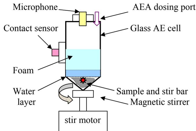
Figure 1. Components of an AFIT<sup>TM</sup> test cell used to measure FI values of eight CCA’s.
