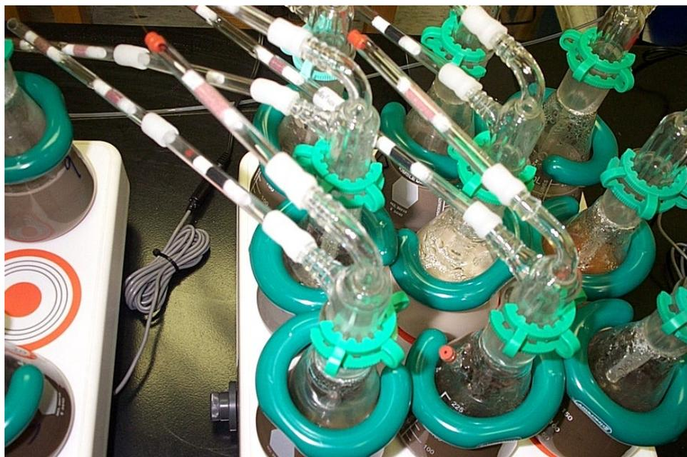
Figure 1. Microbiologically mediated mercury vapor-phase collection apparatus.
