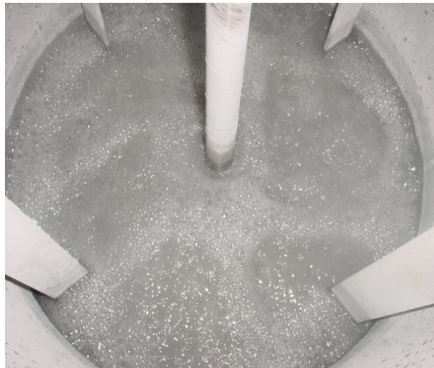
Figure 7: Agitation achieved with pilot rig
