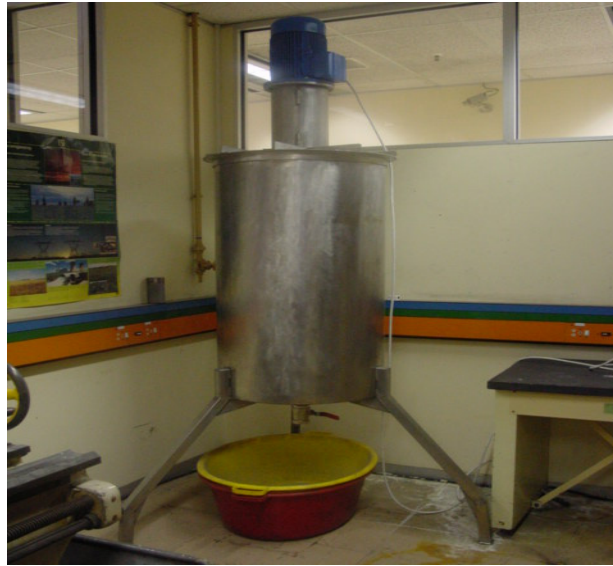
Figure 6: Pilot scale mixer with 250 L tank capacity and turbulator/aeration unit.
