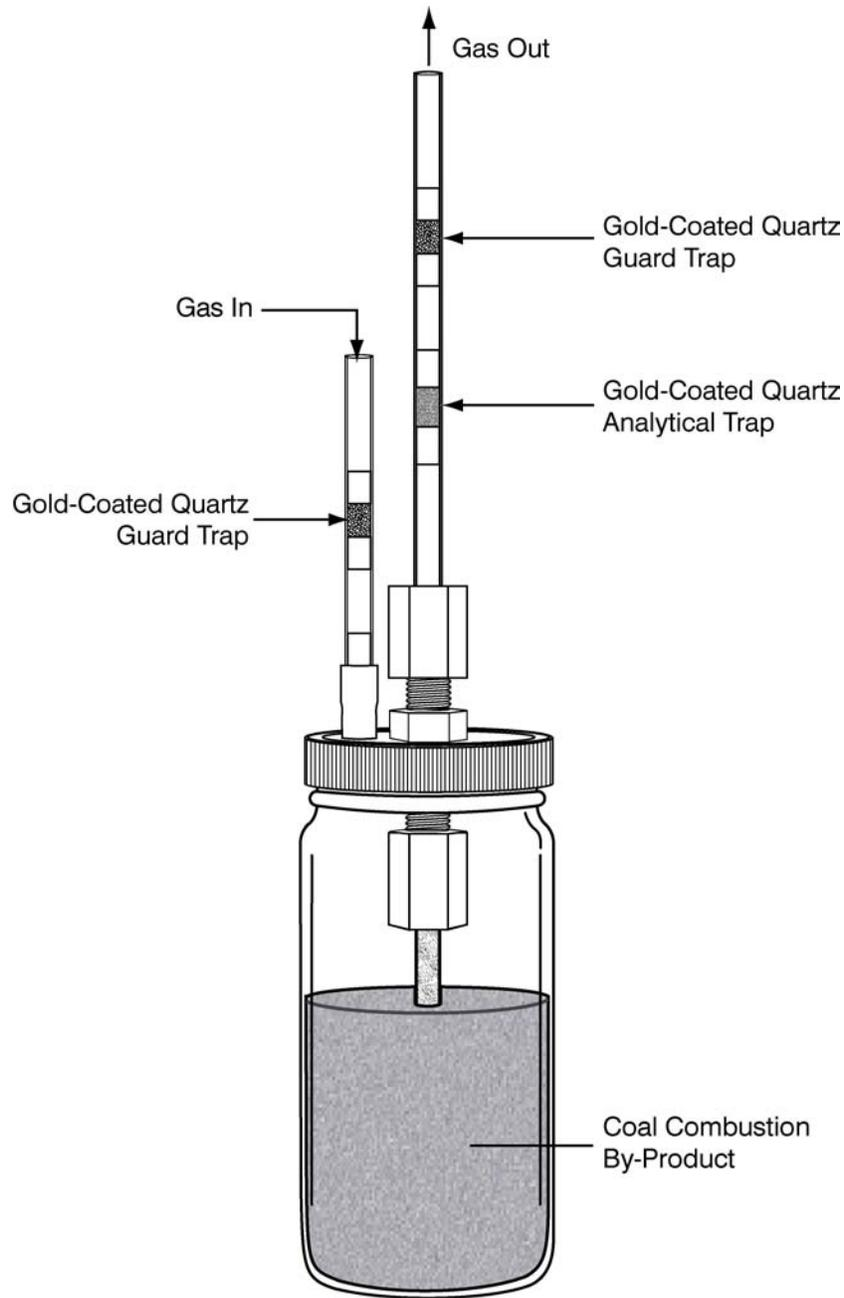
Figure 1. Mercury vapor release collection apparatus.
