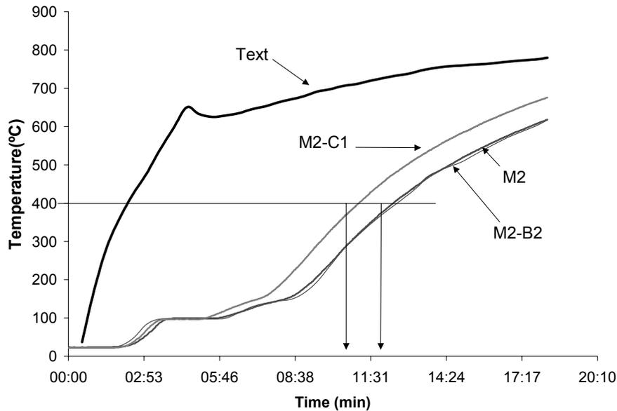
Figure 4. Measurement of the insulating capacity of mortars with vermiculite.
