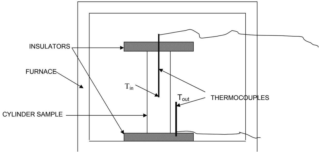
Figure 1. Experimental set up for fire resistance test.
