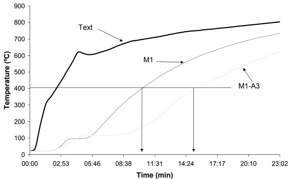
Figure 5. Measurement of the insulating capacity of mortars with MgCl<sub>2</sub>.6H<sub>2</sub>O
