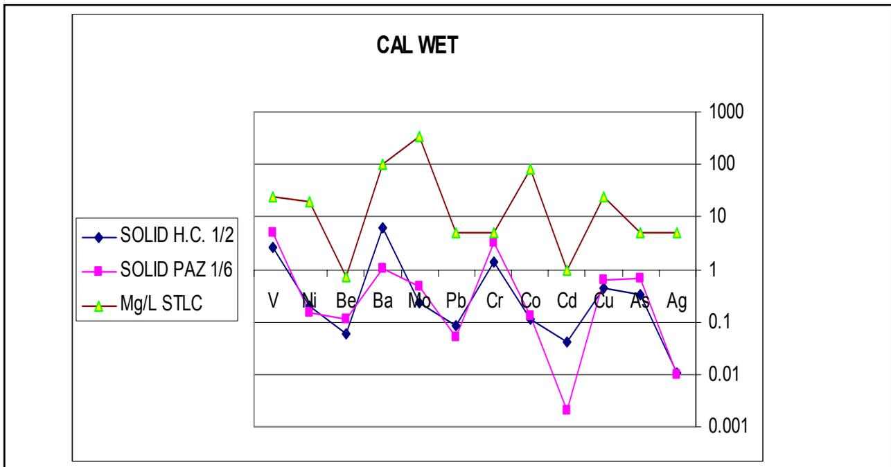
**Figure 2:** Leaching tests of the 1/2 ratio HC/SAFA and 1/6 ratio of PAZ/SAFA using the CALWET method
