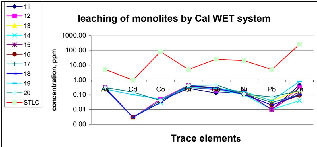
**Figure 3:** Photographs of the Monoliths and the CALWET test results for the grinded monoliths\* (in brackets- the % of sand substitution)
