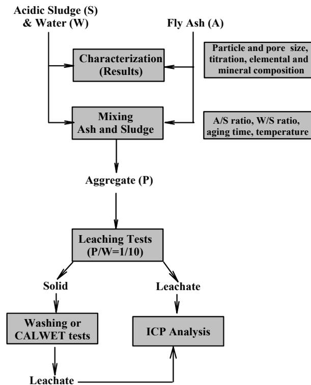
**Figure 1:** General flow sheet used for scrubbing experiments
