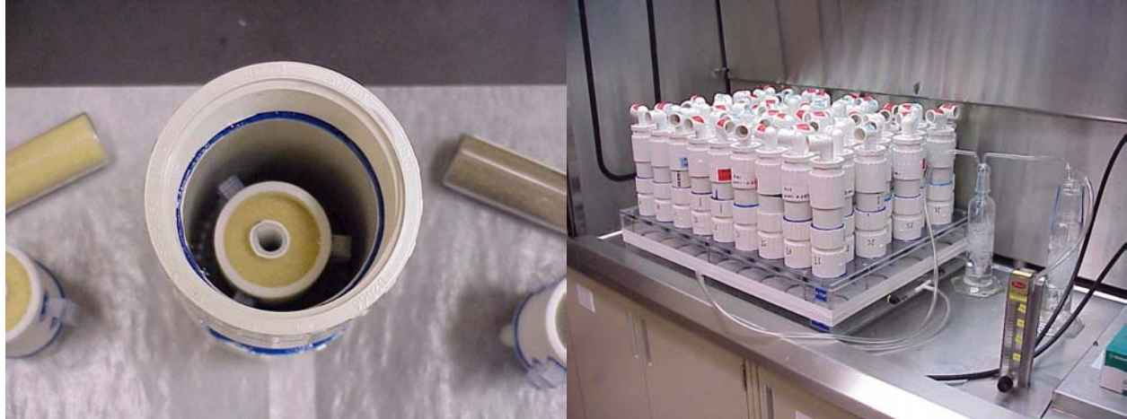
Fig. 2. Experimental apparatus for intermediate-scale humification experiments consisting of porous-walled reactor filled with smectite coated sand (left) and mounted on gas manifold (right) for control of moisture and redox conditions.
