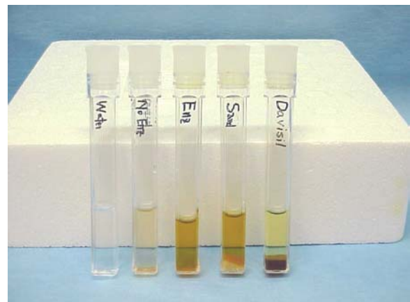
Fig. 4. Batch humification experiments in 7.5-mL cuvettes after three days of contact. Treatments (l to r) water control, monomer with no enzyme, monomer with enzyme, quartz sand in monomer with enzyme, and Davisil in monomer with enzyme.
