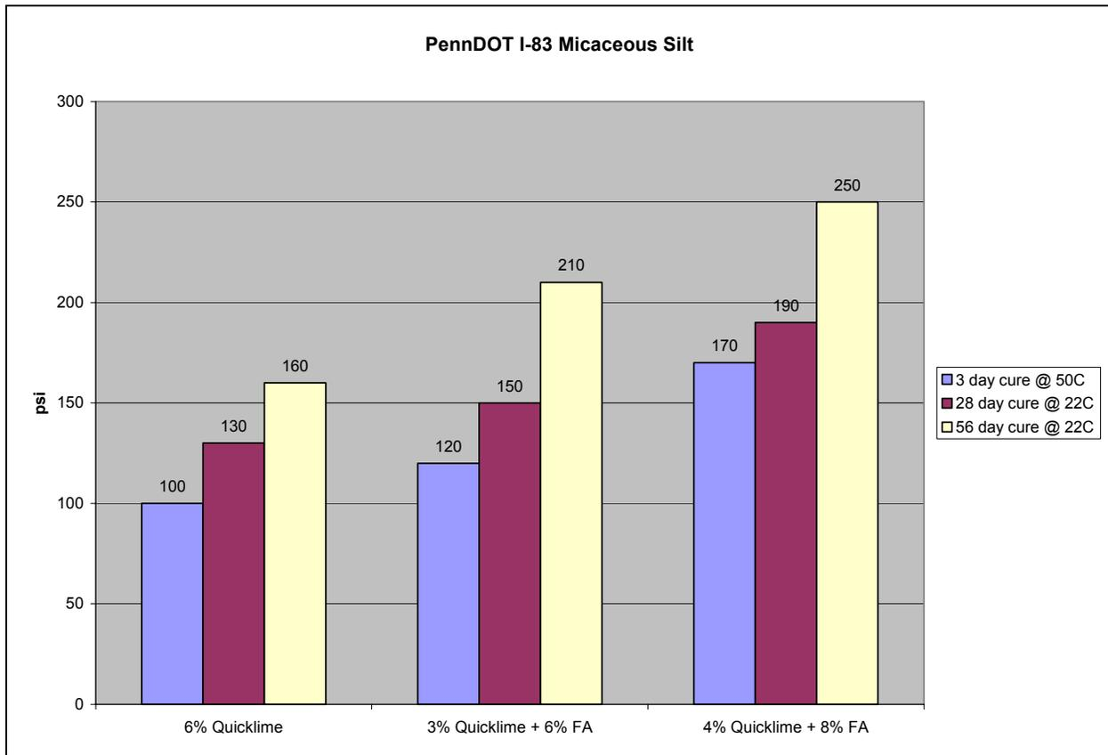
**Figure 4: Lime and lime-fly ash unconfined compressive strengths.**
