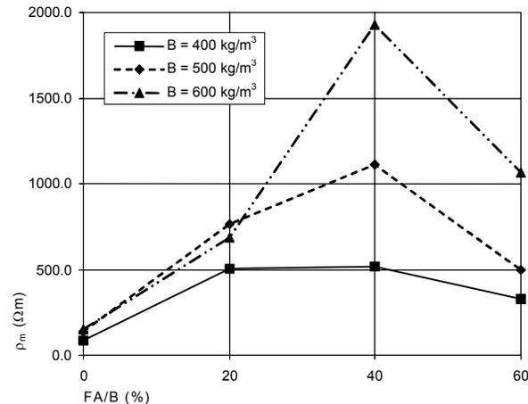
Fig. 4 – Electrical resistivity
