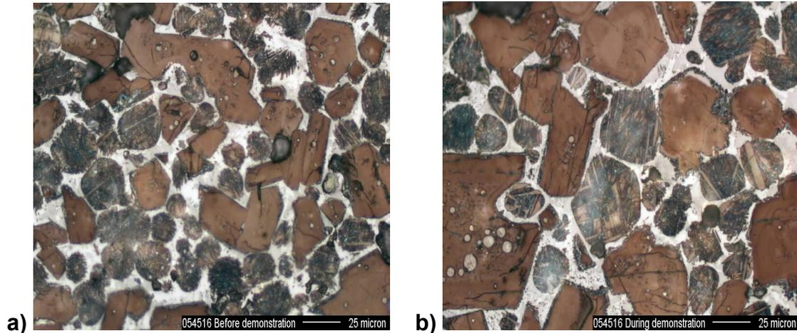
**Figure 3. Photomicrographs of a) clinker before demonstration (without fly ash), and b) clinker produced during demonstration (with fly ash).**
