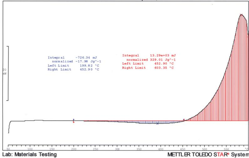
**Figure 1. DSC Plot of Coffeen Fly Ash Sample**
