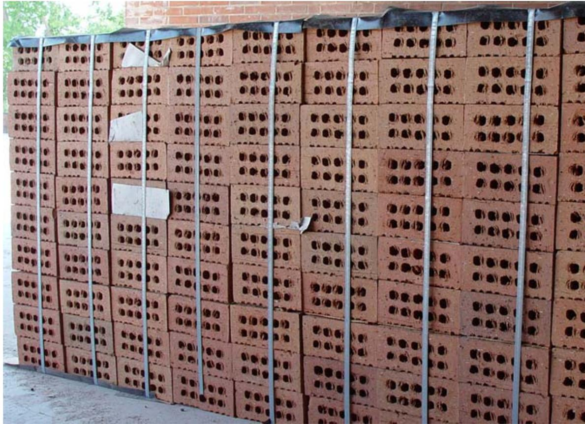
Ten-hole building bricks with 20 wt% fly ash
