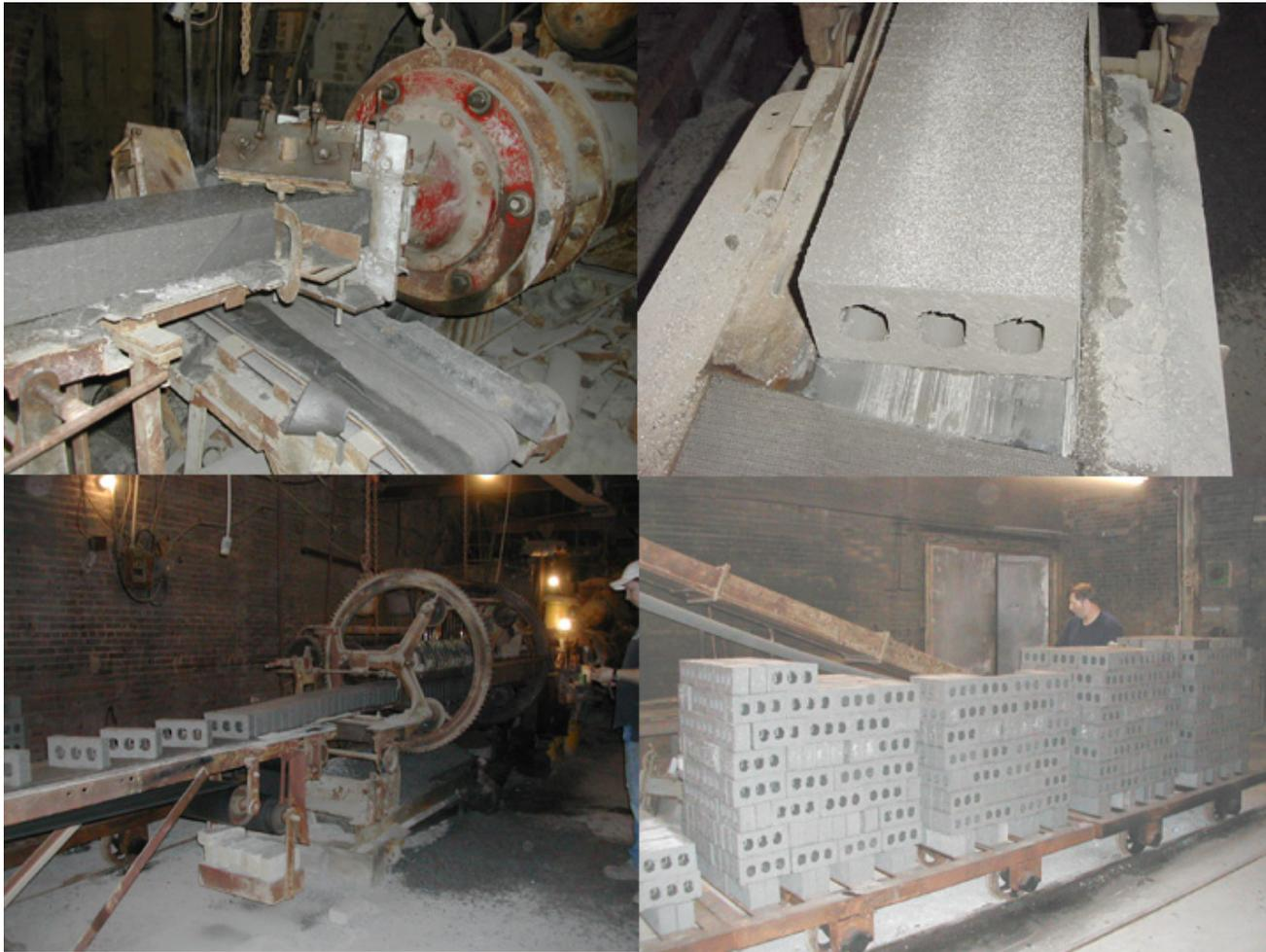
Commercial-scale extrusion test run producing three-hole green bricks
