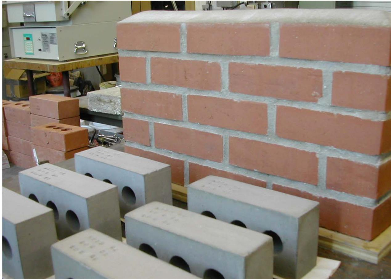
Test wall built using fired bricks from pilot plant production
