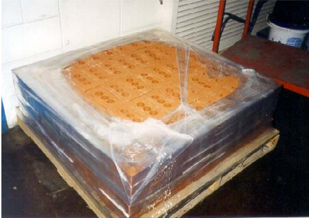
Successful firing of green bricks, containing 40 wt % fly ash,
