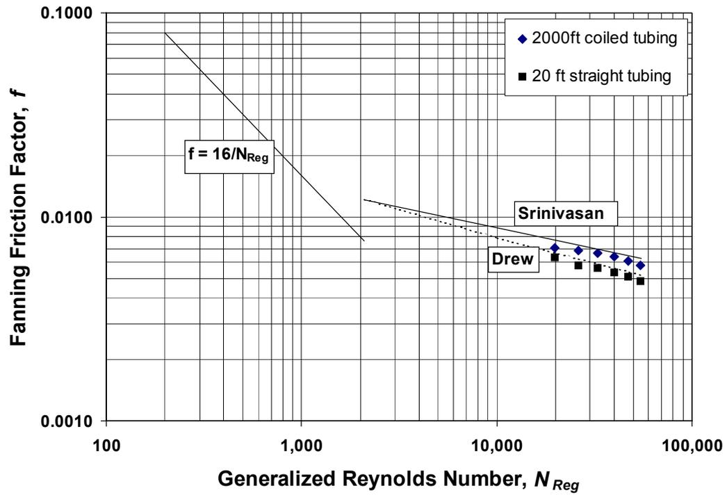
Fig. 5 – Fanning friction factor versus generalized Reynolds number of the Muskogee fly ash slurry.
