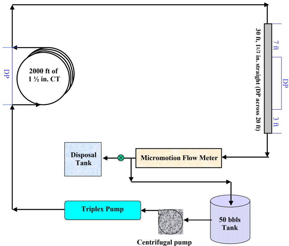
**Fig. 1 – Schematic of experimental setup of flow loop at WCTC, Norman.**
