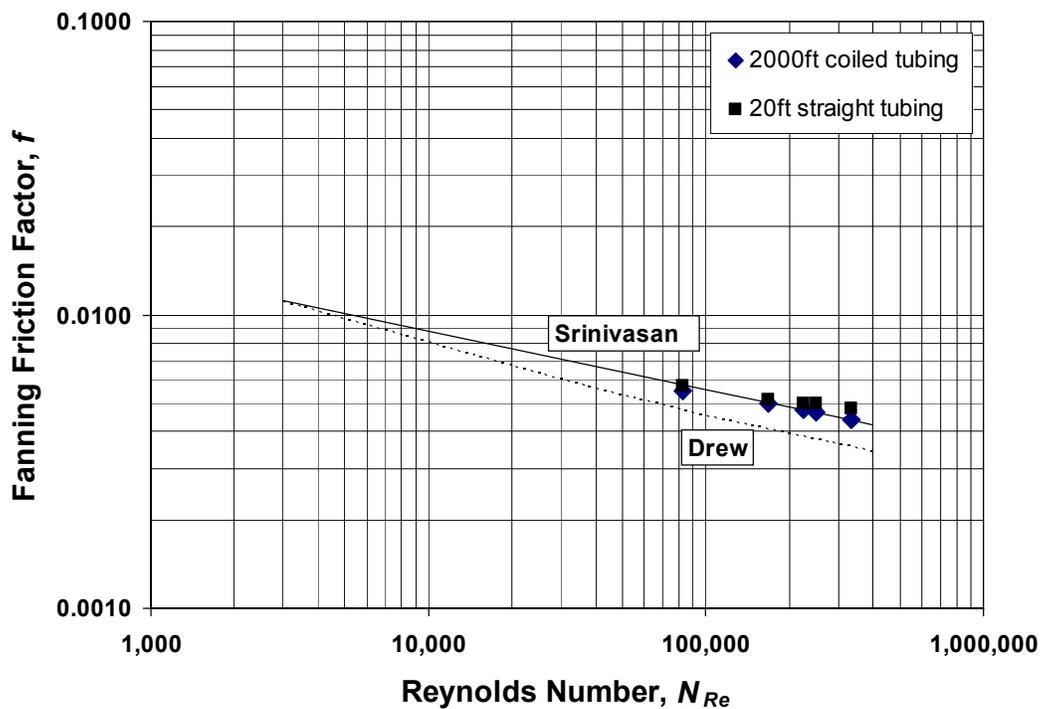
Fig. 4 – Evaluation of water data from coiled and straight 1 ½ in. tubing (pipe ID: 1.188 in., curvature ratio: 0.0165).
