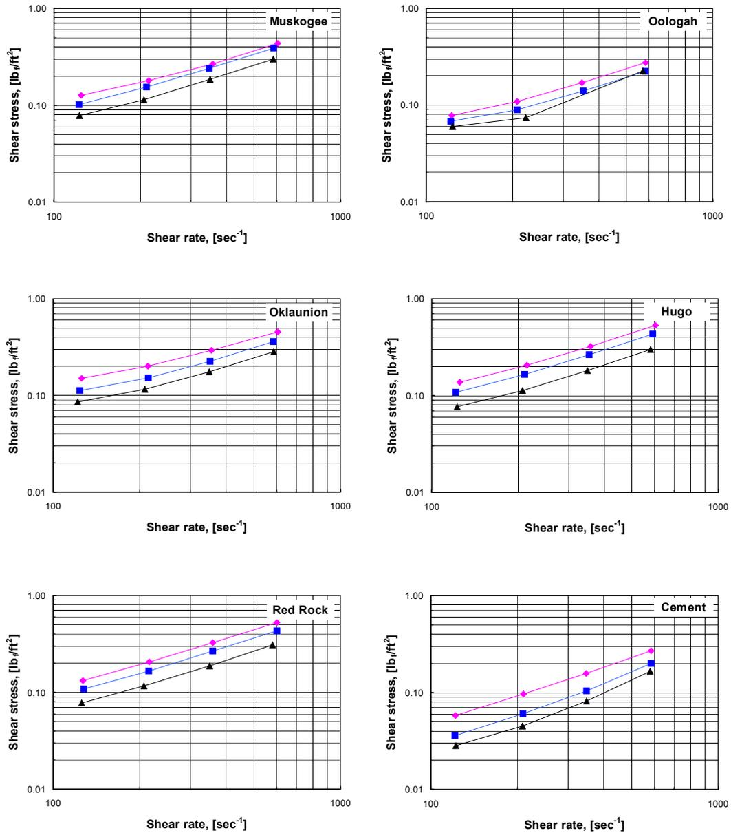
**Fig. 2 – Rheology of fly ash slurries and class H cement slurry at three different temperatures ( $\diamond$ : 80 °F,  $\square$ : 100 °F,  $\triangle$ : 120 °F).**
