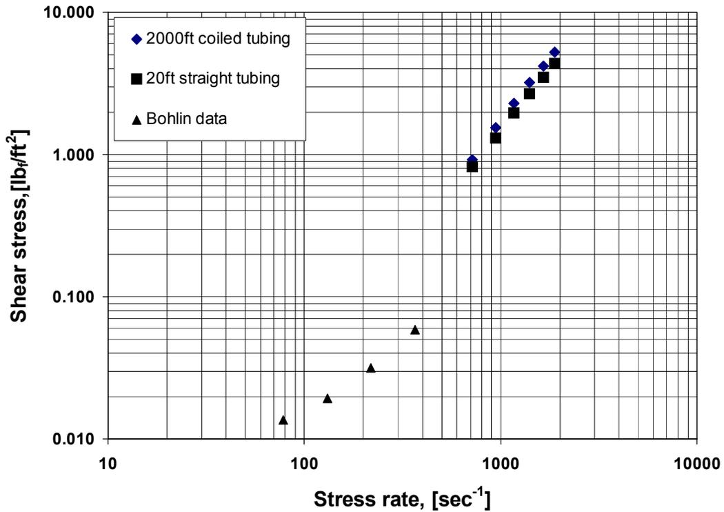
Fig. 3 – Rheogram of the Muskogee fly ash slurry measured by Bohlin rheometer and flow loop system.
