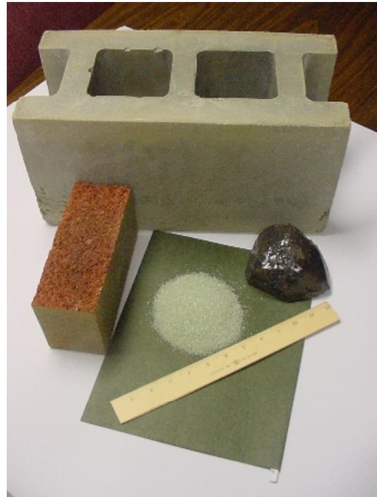
**Figure 4. Glass Recycle Products from the PEM™ System**
