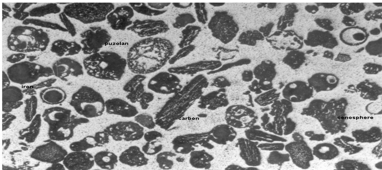
Fig 1. A typical view of fly ash by-products.
