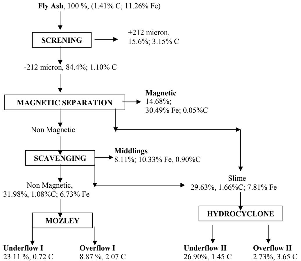
Fig. 2. Optimum flowsheet for separation of fly ash by-products.
