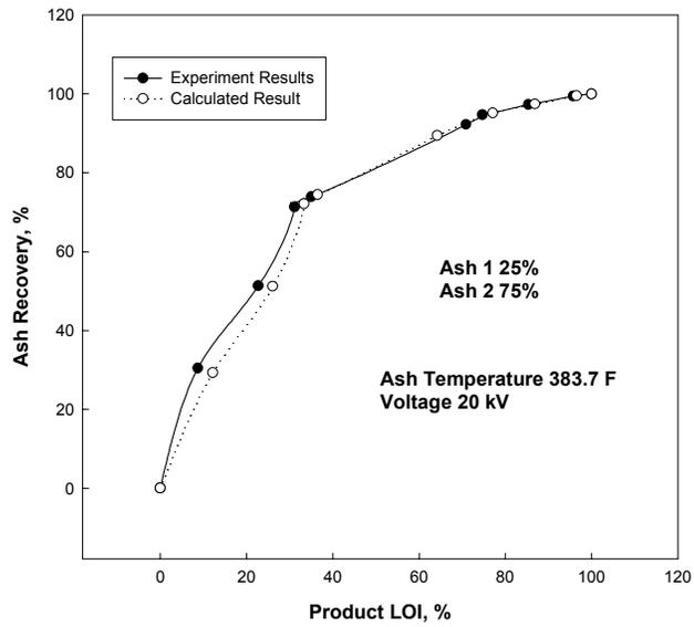
Figure 3. Comparison between experimental results and calculated results
