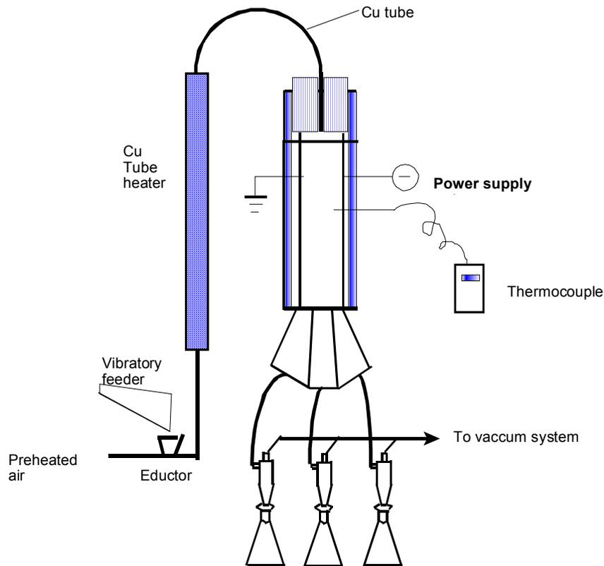
Figure 1. Schematic representation of triboelectrostatic separation system
