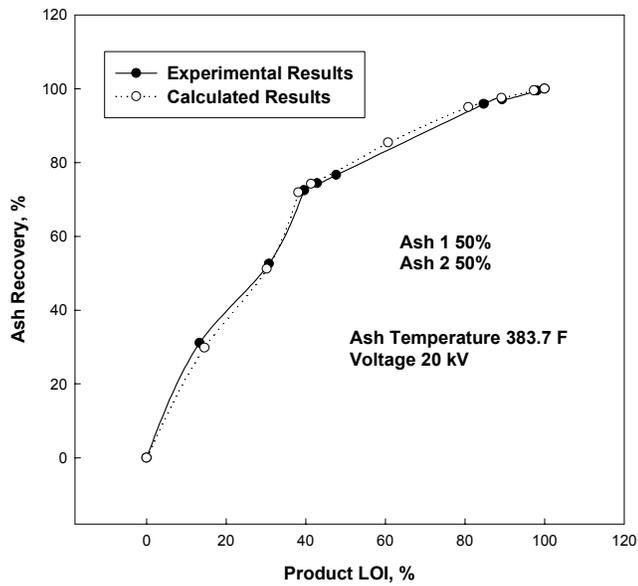
Figure 4. Comparison between experimental results and calculated results
