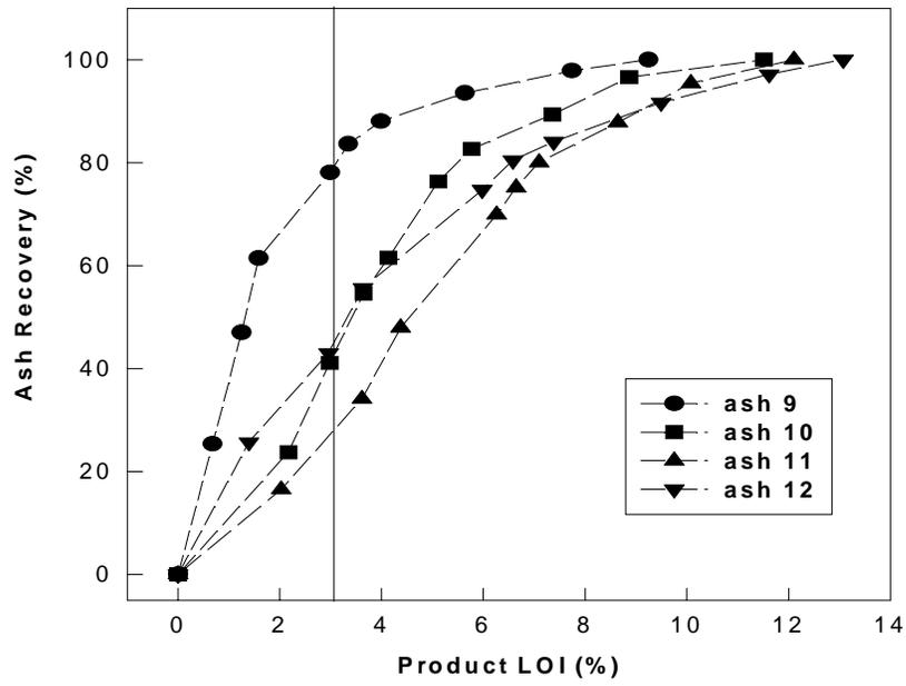
Figure 4. Ash recovery curves for coal combustion fly ashes.
