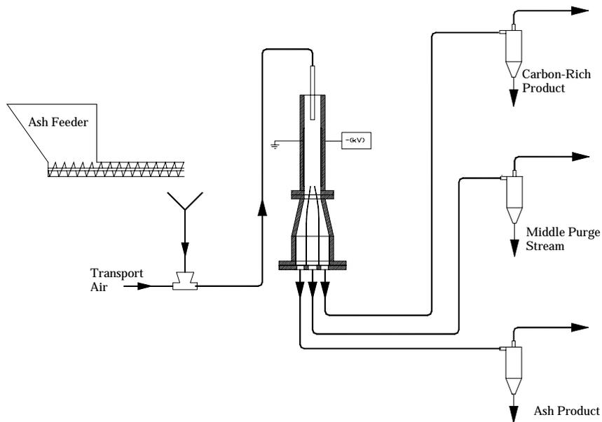
Figure 1. Schematic of continuous feed, bench-scale triboelectric separation system.
