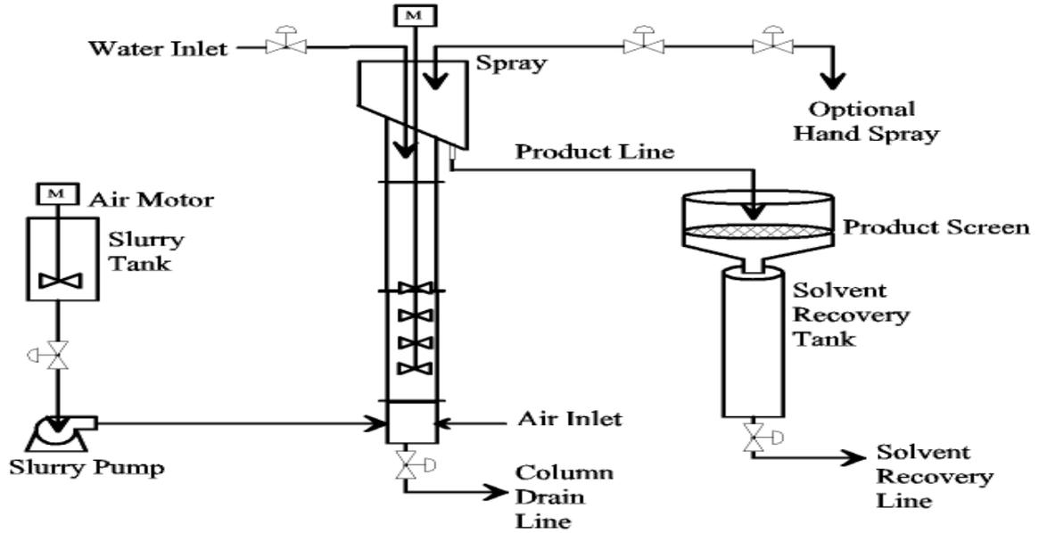
Figure 2 : Agglomeration of Unburned Carbon From FETC Fly Ash Using Various Solvents
