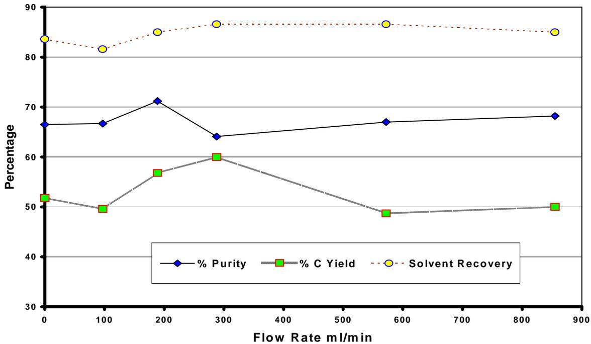
Figure 5: Agglomeration Recovery of Unburned Carbon from FETC Fly Ash at Various Slurry Feed Rates
