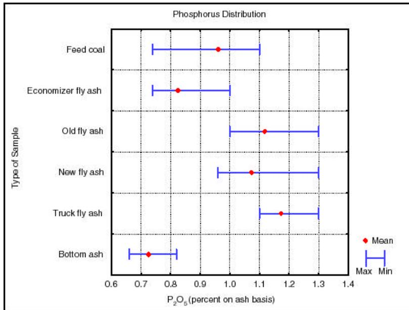
Figure 4. The variation of phosphorus content during the first sampling period. Range plot showing the mean, minimum, and maximum values from the feed coal (n=15), economizer fly ash (n=15), old fly ash sampler (n=11), new fly ash sampler (n=9), truck fly ash (n=11), and bottom ash (n=15).
