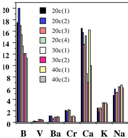
Figure 3: The effect of temperature at 21 ,23 and 34°C on Colombian fly ash with the TCLP method L/S=20
