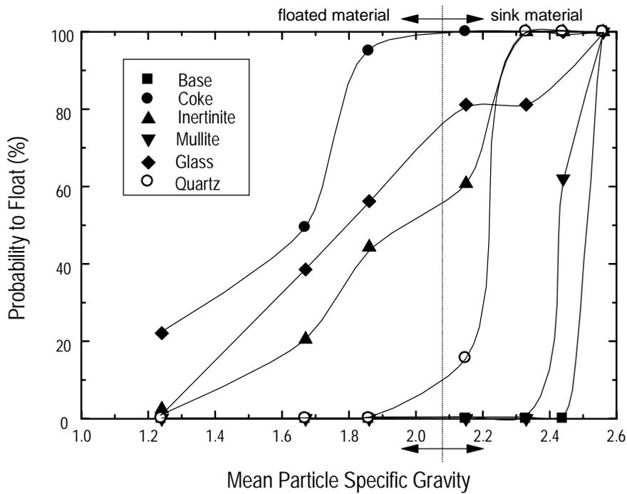
Figure 1. Partition curves on the basis of the mean particle density for each of the petrographic components found in a PCC fly ash. The line represents a hypothetical separation for reducing the carbon content of a high carbon fly ash.
