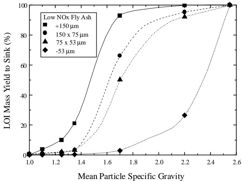
Figure 2. Particle size-by-size particle density distributions of the LOI (i.e., combustible) material in the low NO<sub>x</sub> fly ash sample which show an increase in particle density with decreasing particle size
