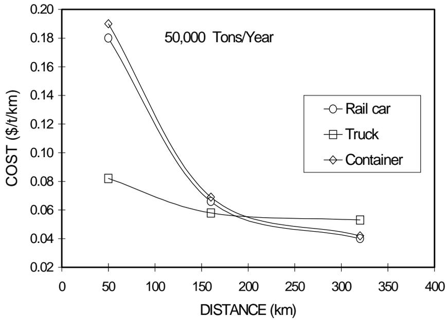
Figure 3. Unit costs in the transportation of 50,000 tons of product by three different systems
