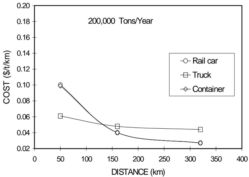
Figure 4. Unit costs in the transportation of 200,000 tons of product by three different systems
