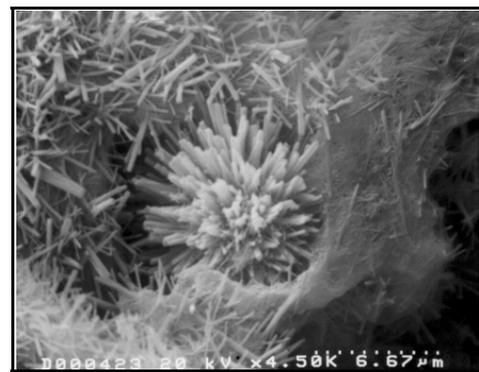
Fig. 8. View of ettringite in AFBC subgrade
