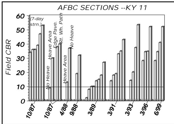
Fig. 7. Field CBR values over a 12-year span.
