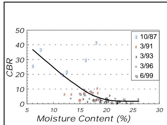
Fig. 6. CBR as a function of moisture content
