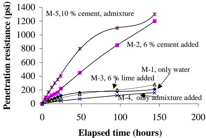
Figure 4: Penetration Resistance vs. Time for Modified Mixes
