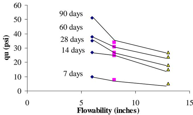
Figure 1: Unconfined Compressive Strength vs. Flowability
