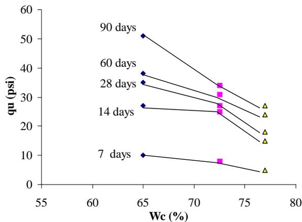
Figure 2: Unconfined Compressive Strength vs. Water Content
