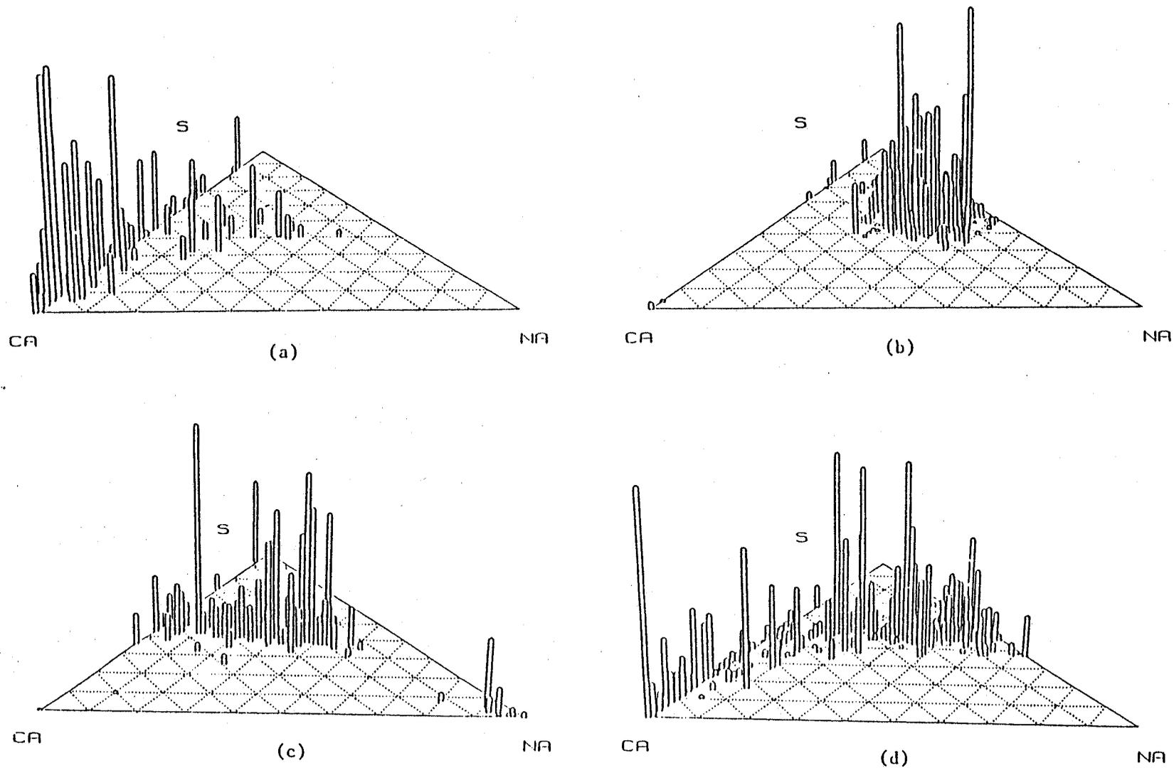
Figure 3. Ca-Na-S volume frequency-ternary plots for Beulah lignite ash from: (a) UA combustor, Imp. 1 + cup; (c) UA combustor, Imp. 2 + 3 + 4; (b) UA combustor, Imp. 5-8 + AF; and (d) SECV combustor, electrostatic precipitator.
