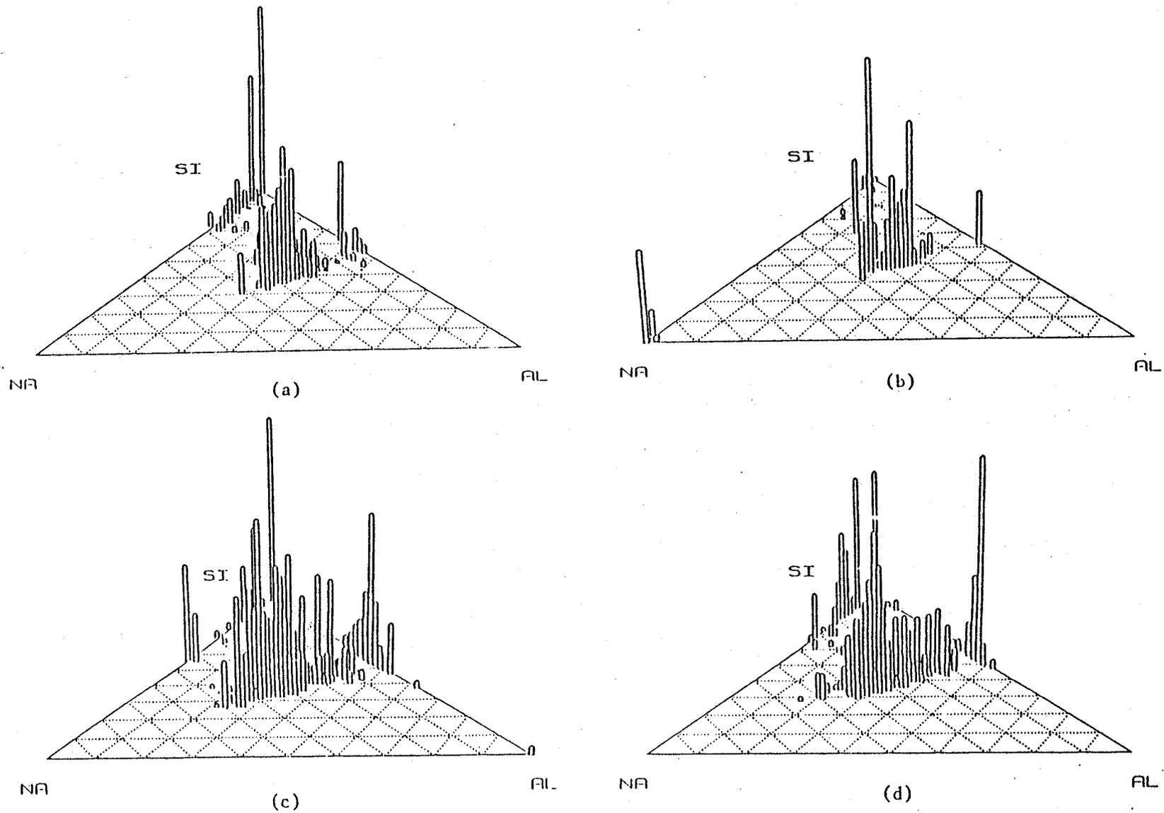
Figure 2. Na-Si-Al volume frequency-ternary plots for Beulah lignite ash from: (a) UA combustor, Imp. 1 + cup; (b) UA combustor, Imp. 5-8 + AF; (c) SECV combustor, combustion chamber; and (d) SECV combustor, horizontal duct.
