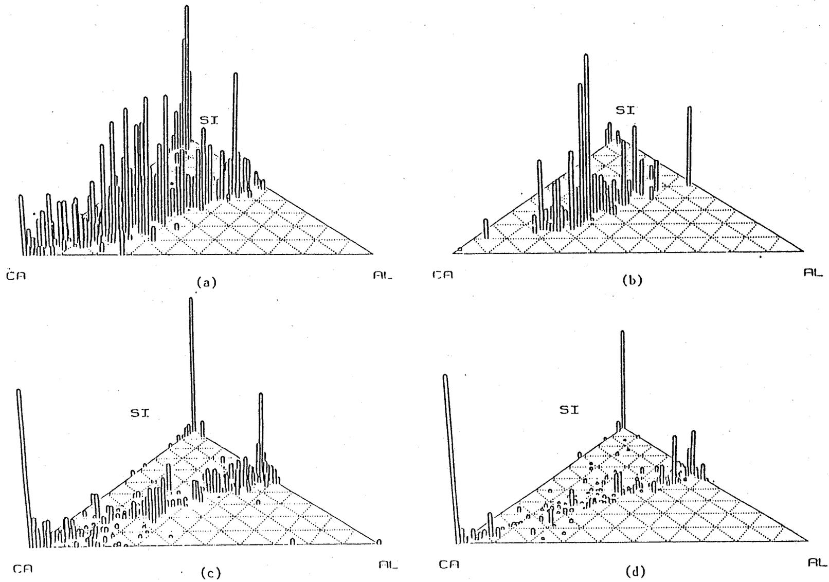
Figure 1. Ca-Si-Al volume frequency-ternary plots for Beulah lignite ash from: (a) UA combustor, Imp. 1 + cup; (b) UA combustor, Imp. 5-8 + AF; (c) SECV combustor, combustion chamber; and (d) SECV combustor, horizontal duct.
